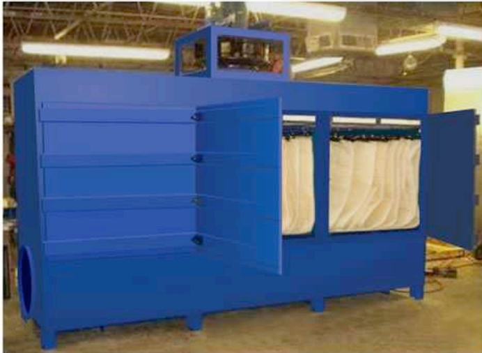
Model HMF-1600-20-H with (4) 40% Pre-Filters, (8) 95% Micro Glass Bag Filters, HEPA Minipleat After-Filter, 20 HP, Rated 13,000 CFM
